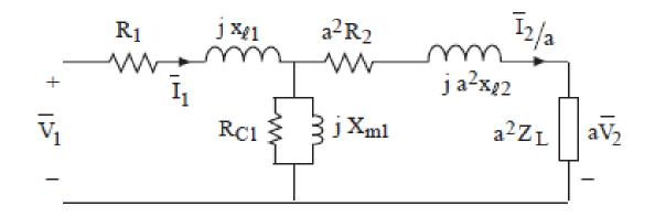
• If we desire a similar equivalent circuit with all quantities referred to winding 2, it can be easily deduced. The impedances are divided by  $a^2$ , voltage is divided by a and the current is multiplied by a.
