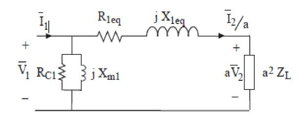
• The equivalent impedances referred to secondary side:
