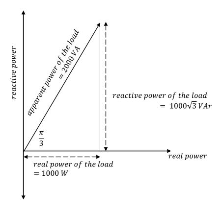
(ii) [40 points] Assume that the source power factor equals that of the load, and there are no other elements in the circuit. Under these conditions, with the power factor maintained at its specified value determined in (i), determine the amount of additional load in W of the real power that the source can supply without the violation of its 3,000–VA rating.
