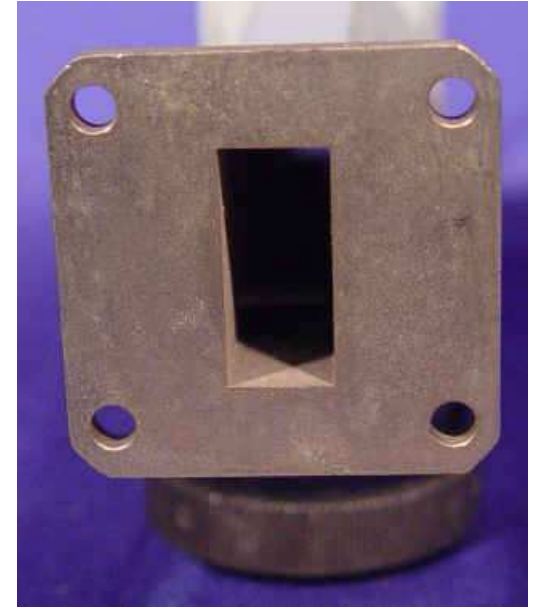
2.29 cm by 1.012 cm Standard X-band (8.2-12.4 GHz) waveguide in which only TE 10 mode is non-evanescent within X-band.
