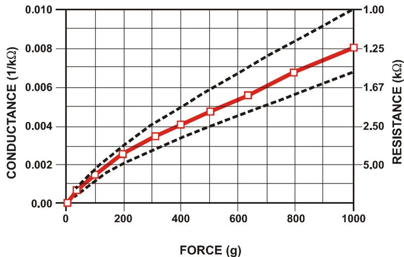
Figure 5.1: Empirical Force-Resistance curve of our chosen FSR
