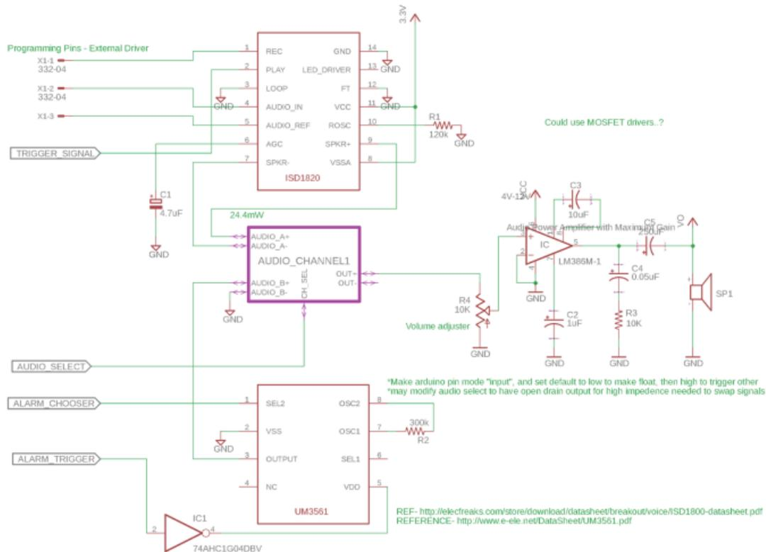
Figure 3.1: Audio Circuit Schematic
