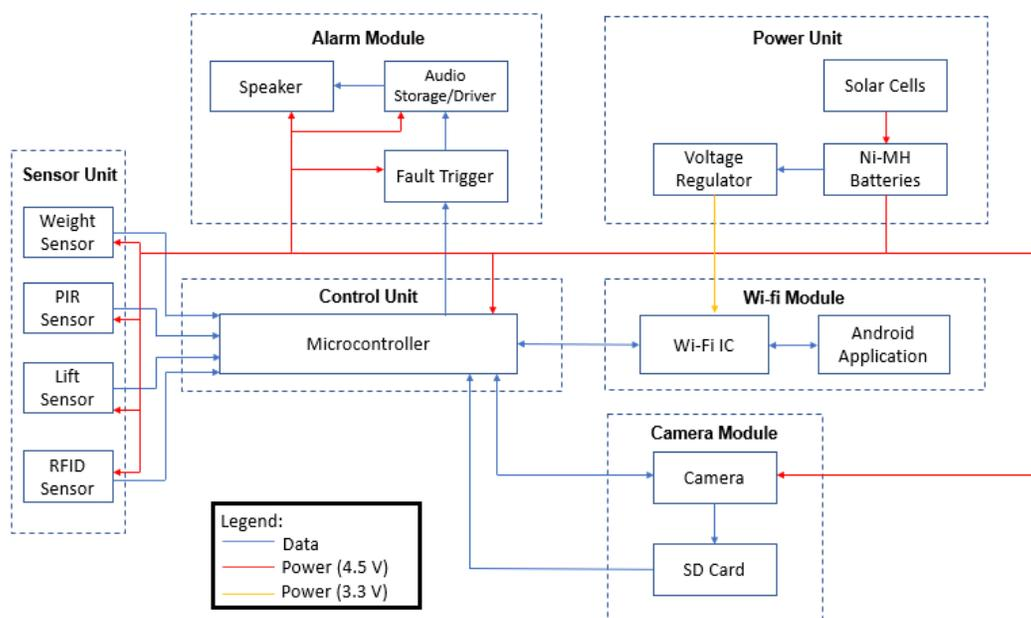
Figure 2.1: Block Diagram
