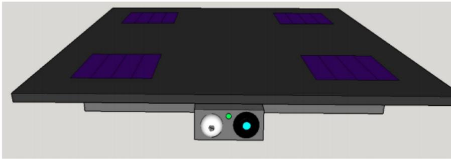
Figure 2.2: Top angle view showing solar cells, camera, and PIR sensor
