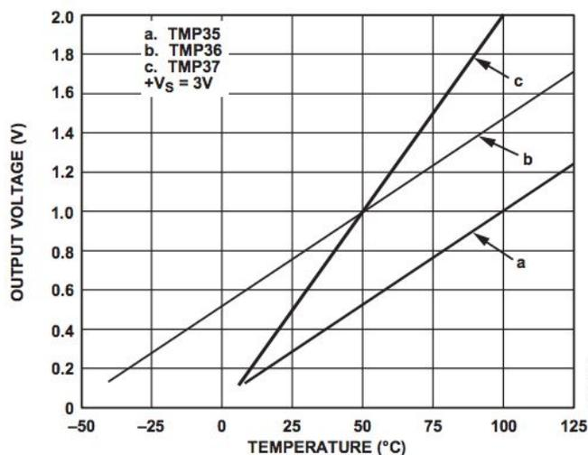
Fig. 7. Temperature Sensor Characteristics[15]
