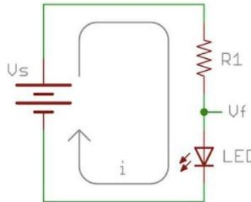
Fig. 8. Current-limiting Resistor Example
