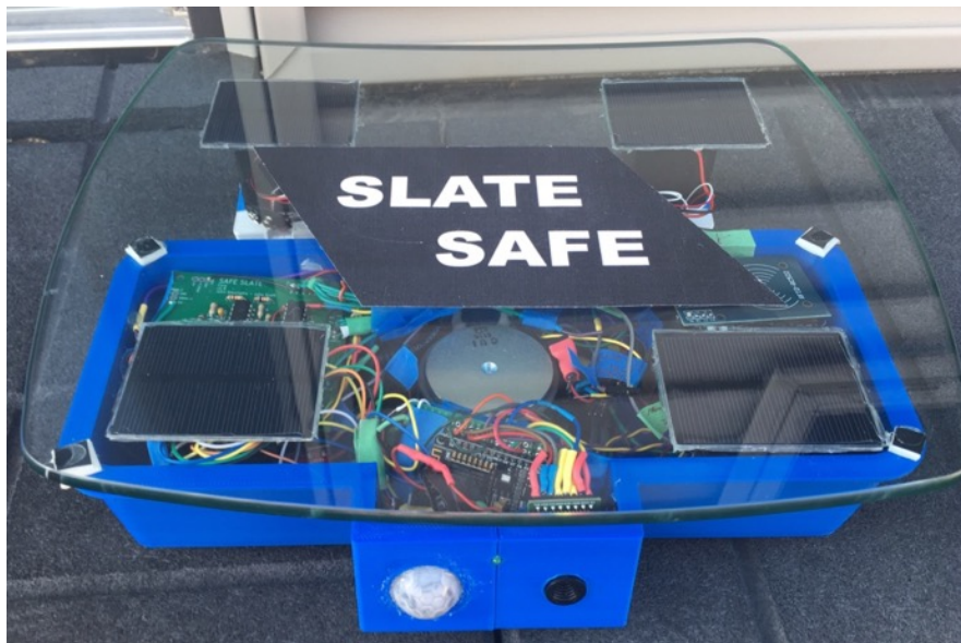
Figure 1: Slate Safe theft deterrence system.
