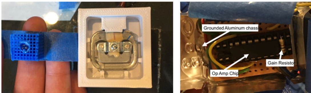
Figure 8: To the left is the load cell housing with the 3D printed buffered foot. To the right is the instrumentation amplifier circuit inside a grounded chassis.
