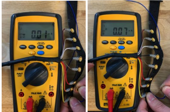
Figure 13: Current Measurement (Left:DC, Right:AC)
