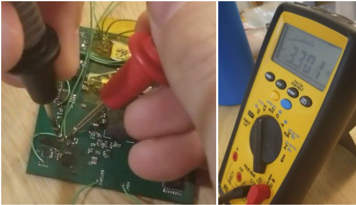
Figure 21: Battery Through TPS62740 Buck Converter Supplying Constant 3.3V
