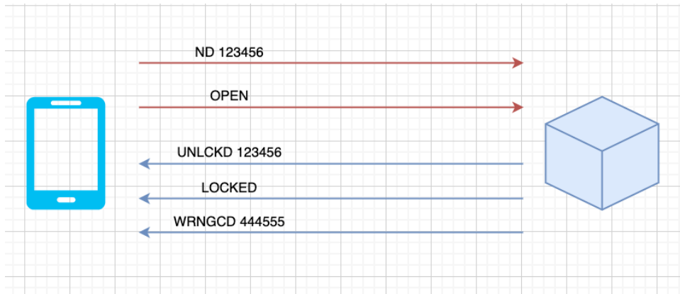
Figure 5: TCP communication between the devices
