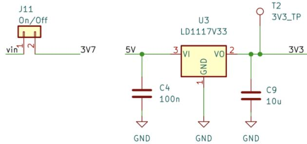
Figure 2.3.1.1 Linear Voltage Regulator
