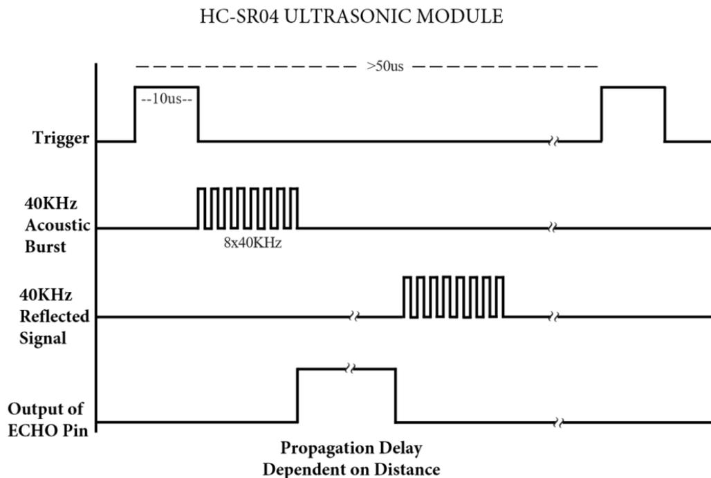
Figure1: Representation of trigger signal scountic bursts, reflected signal and output of ECHO pin (HC-SR04)
