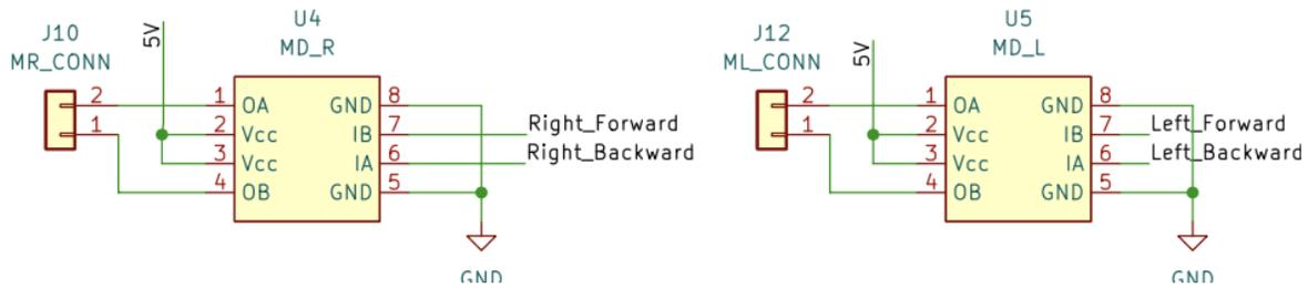
Figure 2.3.4.1 Motor Driver Schematic
