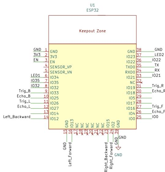
Figure 2.3.2.1 Esp32 Schematic
