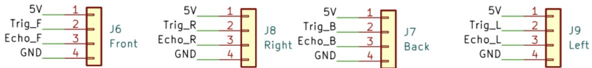
Figure 2.3.3.1 Ultrasonic Sensors Schematic
