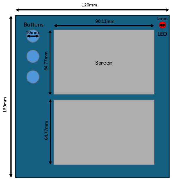
Figure 3: Physical dimensions of the JargonJolt
