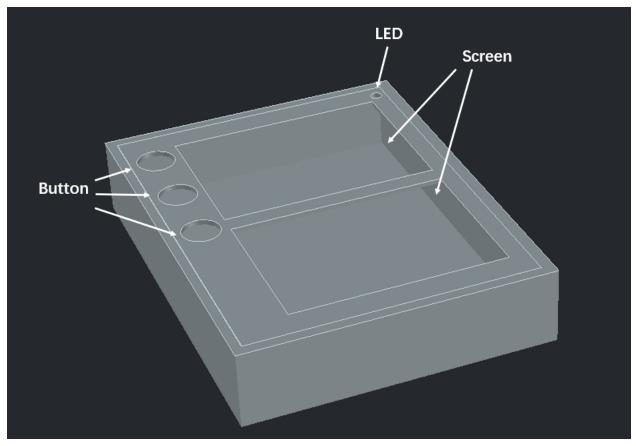
Figure 4: CAD representation of the JargonJolt physical design
