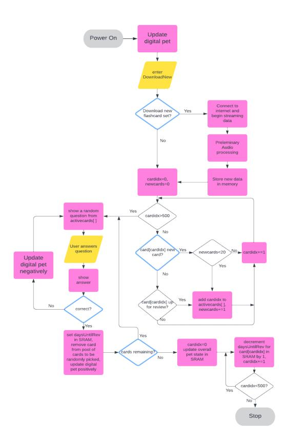
Figure 5: High level MCU algorithm flowchart
