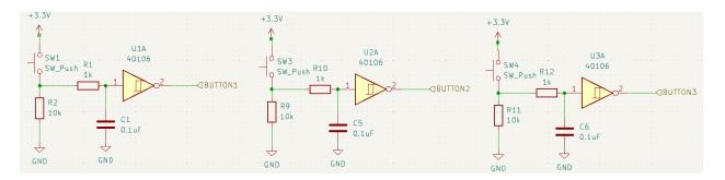
Figure 7: Schematic of face buttons
