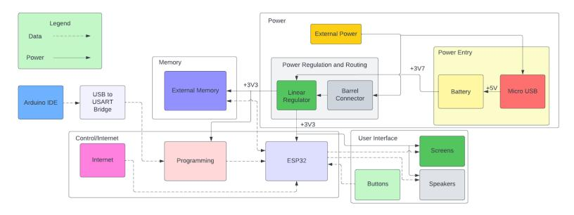
Figure 2: High level block diagram for JargonJolt
