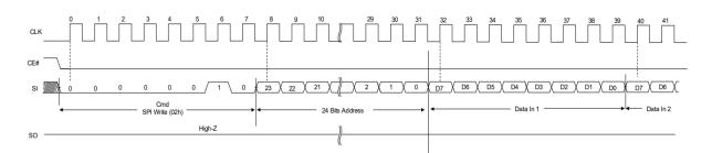
Figure 9: Timing diagram for writing to IS66WVS4M8ALL
