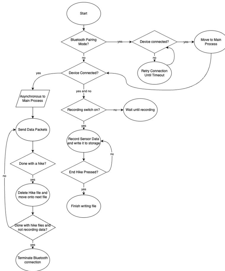
The software outlined in the flowchart is designed for managing sensor data recording and Bluetooth connectivity for a hiking activity tracker. It begins by determining whether it should be in Bluetooth pairing mode. If so, it checks for a connected device and, if not found, enters a retry loop until a timeout is reached. Once a device is connected, the software transitions to the main process.
