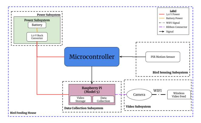
Figure 2: Block Diagram of Design
