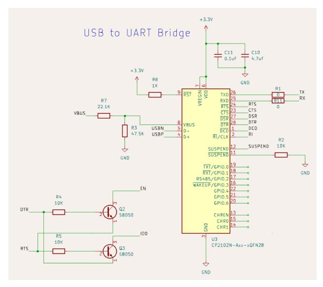
Microcontroller and USB to UART Bridge's Schematic
