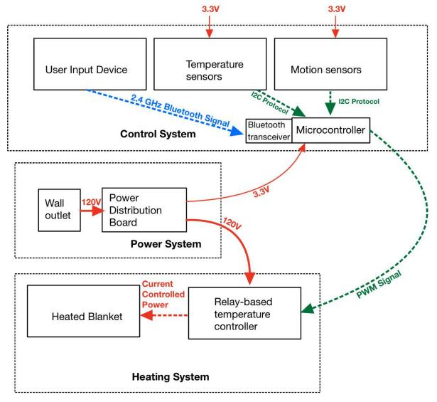
Fig. 2. Block diagram of our overall design.
