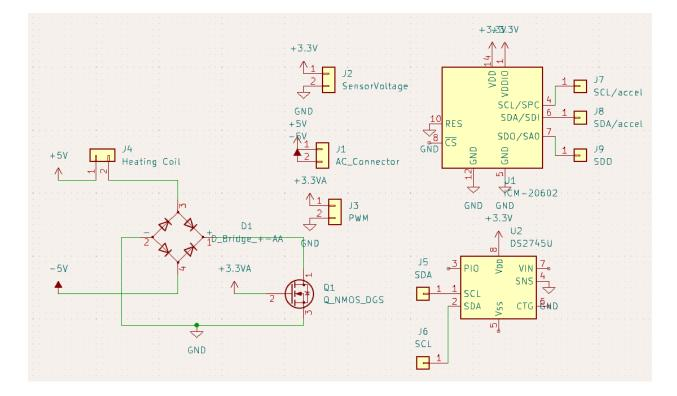
Fig. 5. Schematic for Heating Module in KiCAD.
