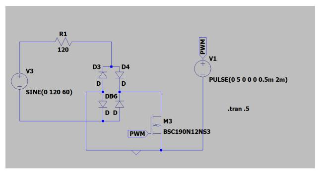
Fig. 4a. AC Pulse Width Modulation circuit using MOSFET.
