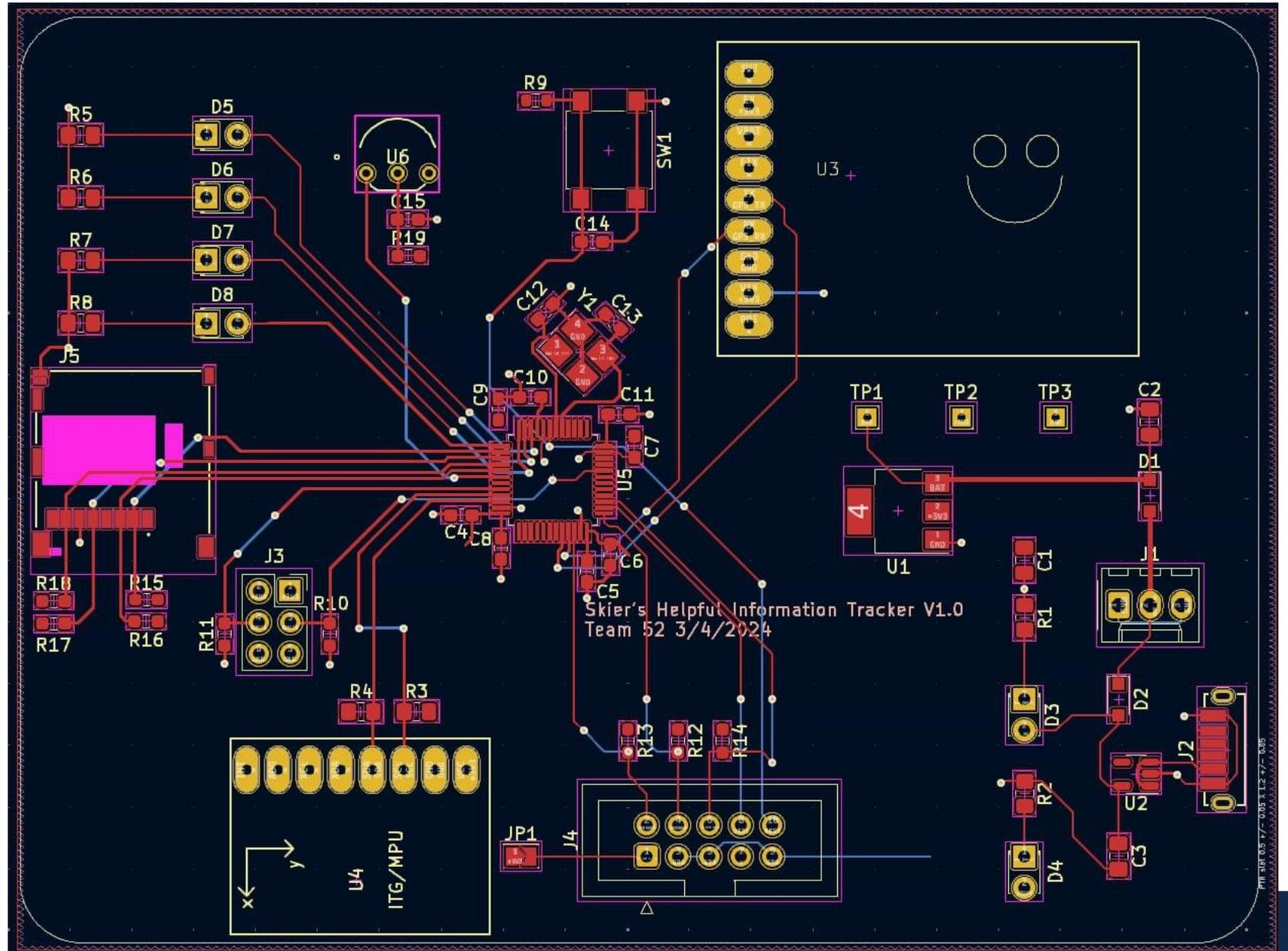
Figure 10: PCB Layout
