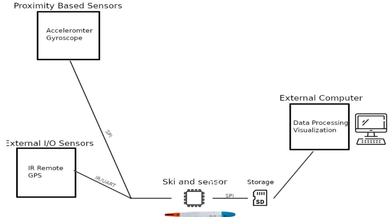
Figure 2: High Level Design
