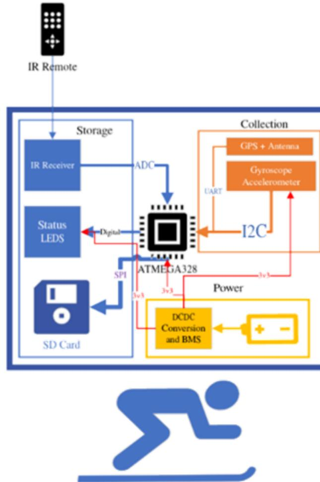
Figure 4: Device Block Diagram
