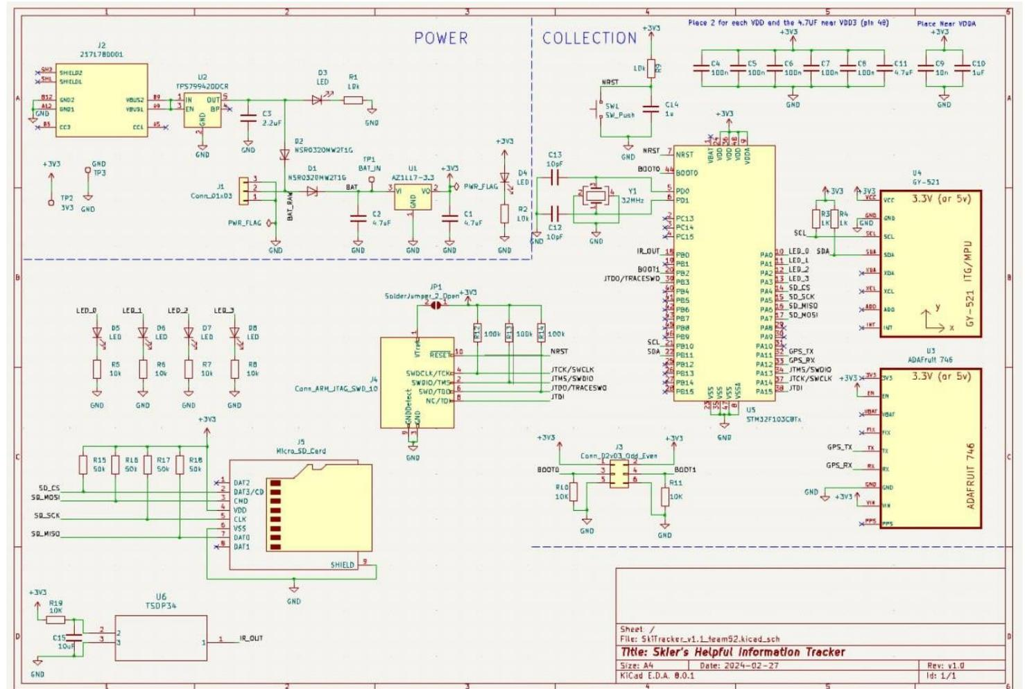
Figure 9: PCB Schematic
