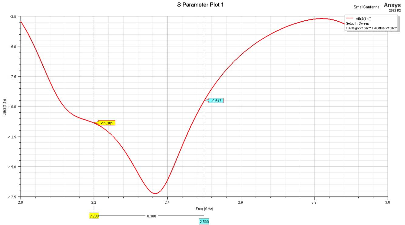
Figure 6: Simulated Antenna Reflection Coefficient From Ansys HFSS
