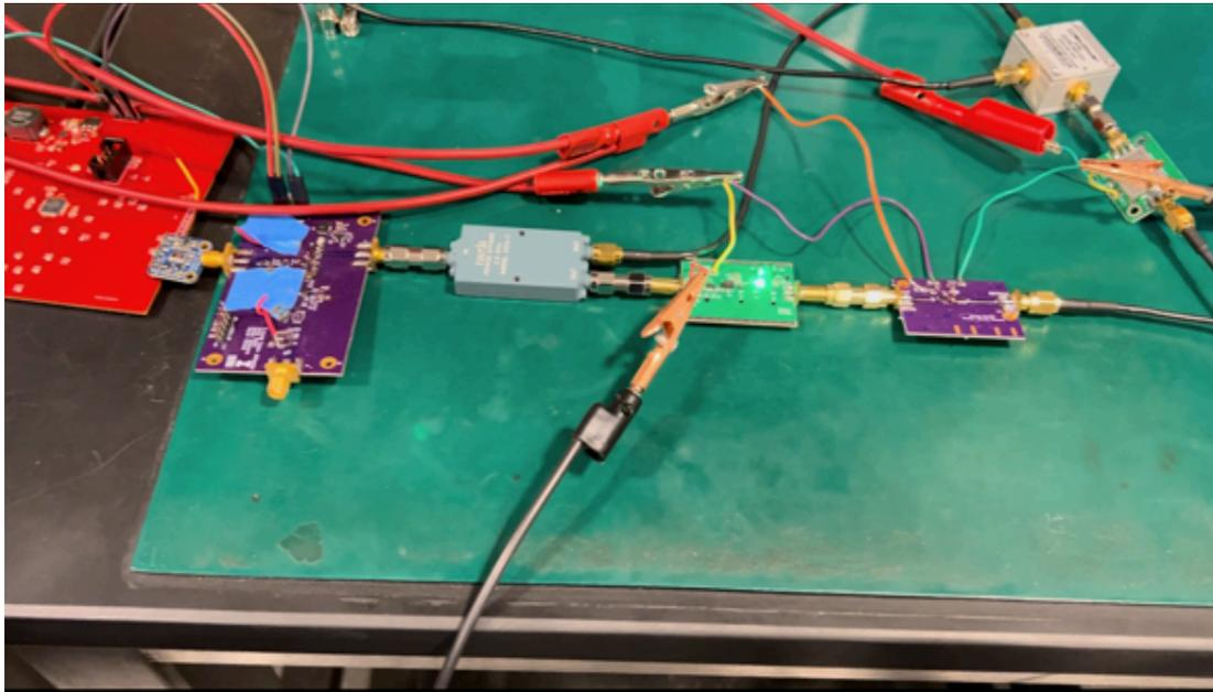
Figure 3: Final System Construction, From Left to Right: Power/Processing Unit, VCO Board, Power Divider, Power Amplifier, LNA, Mixer
