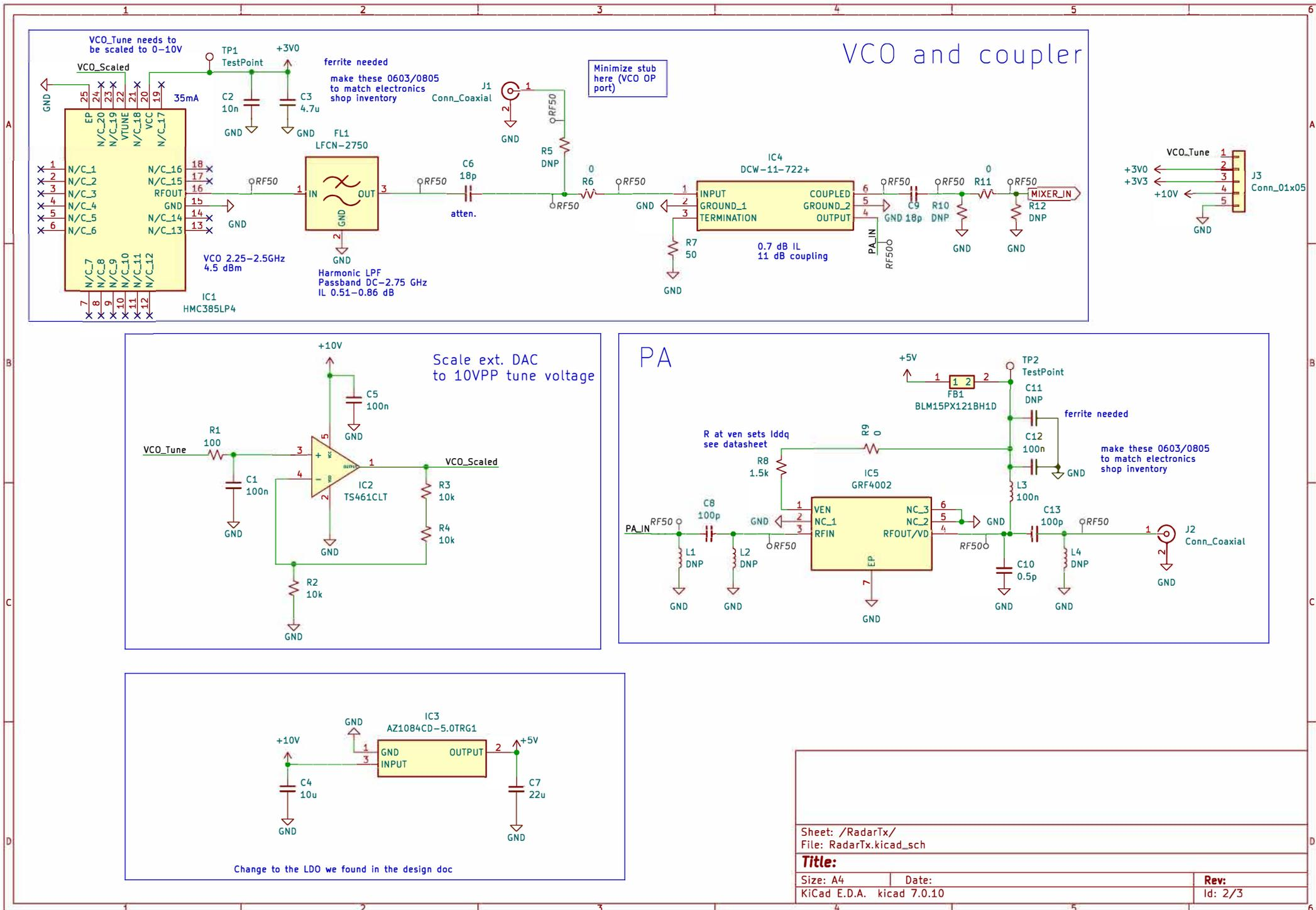
Figure 13: Radar Unit Version 2 Transmitter Schematic - Only the VCO Was Used
