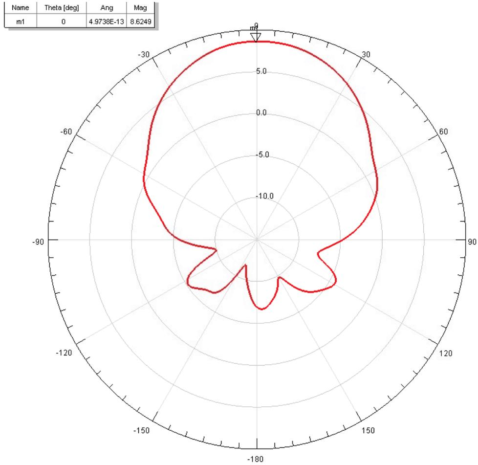
Figure 7: E-Plane Radiation Pattern of Cantenna showing ~8.7 dB of gain
