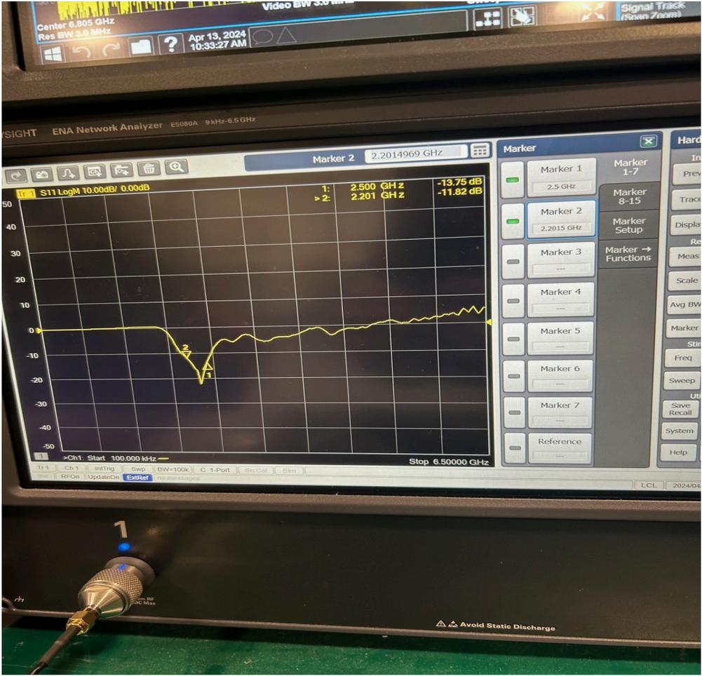
Figure 9: Measured Reflection Coefficient of Cantenna
