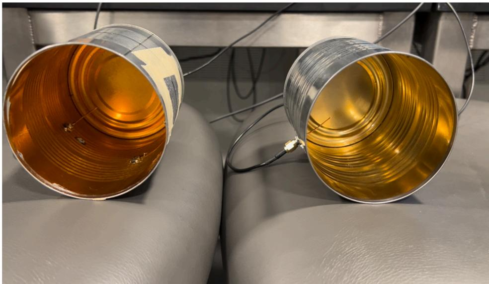
Figure 8: Final Cantenna Design
