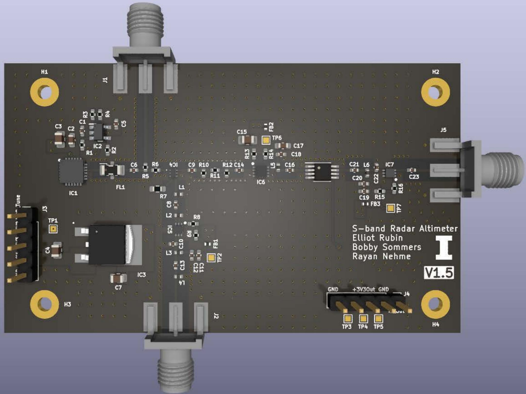
Figure 15: Radar Unit Version 2 Layout
