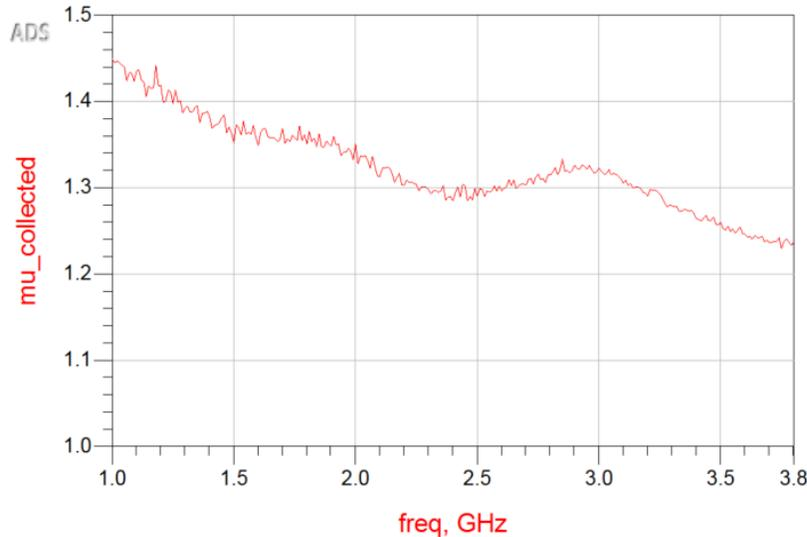
Figure 4: PA/LNA Stability Factor,  $\mu$ , Captured From Network Analyzer and Plotted in ADS
