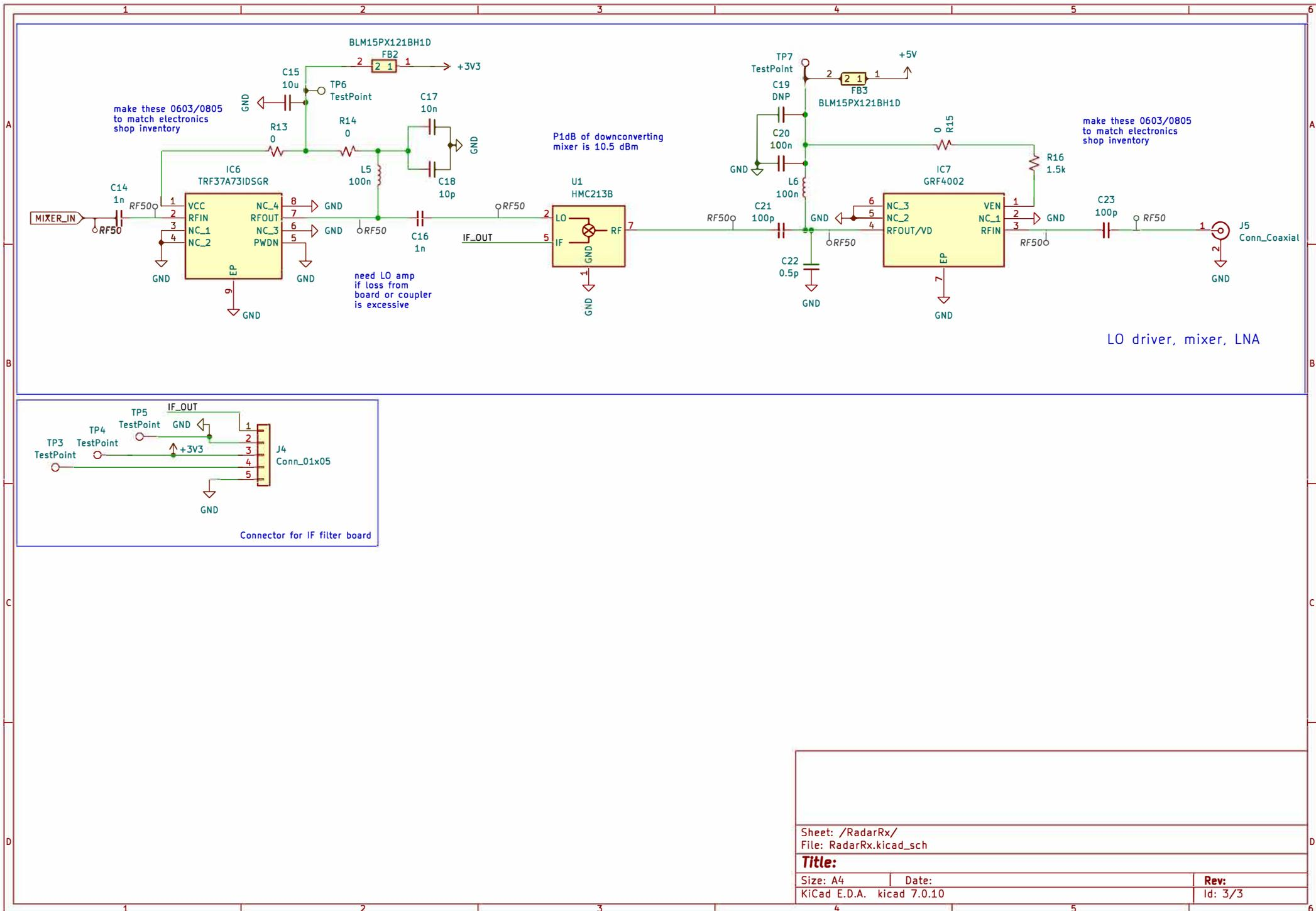
Figure 14: Radar Unit Version 2 Receiver Schematic - Unused in Final Design
