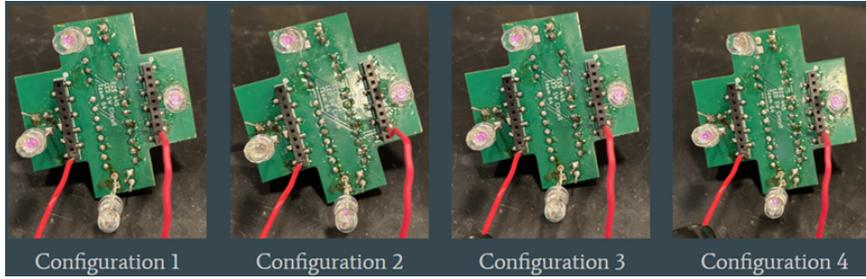
Figure 4: Different configurations of the LED array
