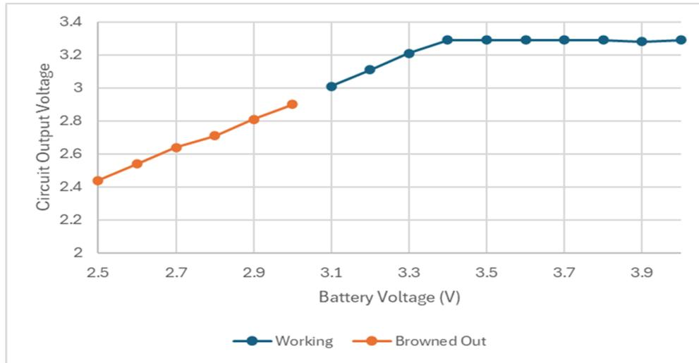
Figure 18: Graph showing the circuit output voltage at various battery levels, highlighting working conditions and brown out occurrences.
