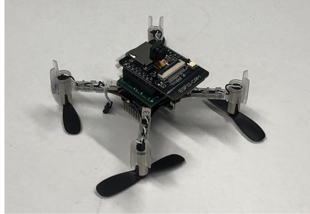
Figure 10: The entire system mounted on the drone, upside down to emphasize the transmission system.
