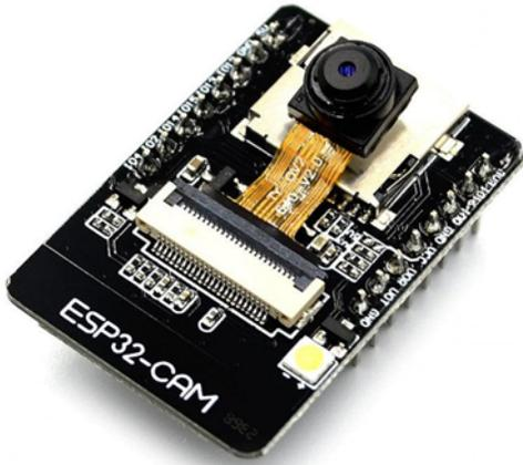
Figure 9: The ESP32-CAM used in the system.
