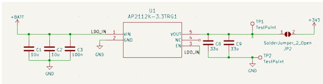
Figure 16: Schematic of the LDO
