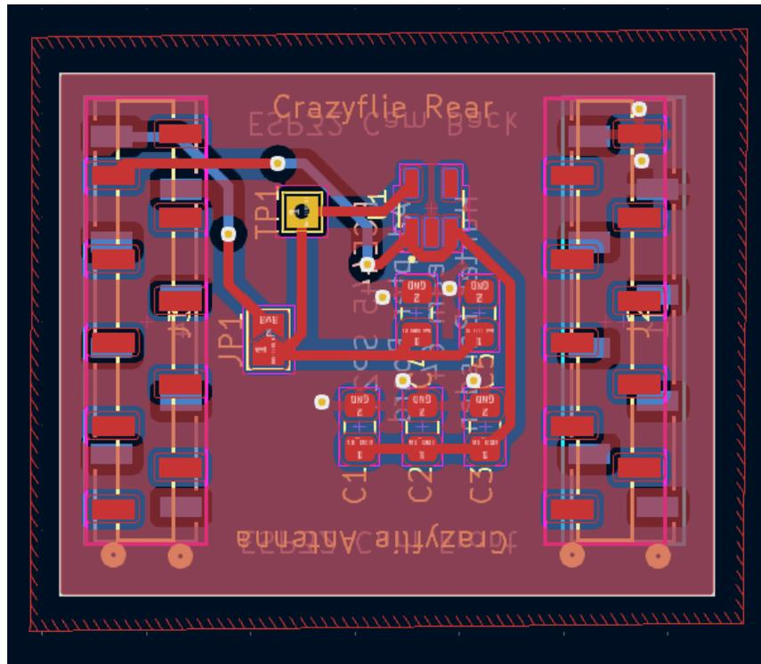
Figure 6: PCB Layout of Adapter Board
