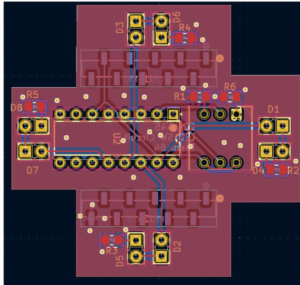
Figure 3: PCB Layout of LED Board
