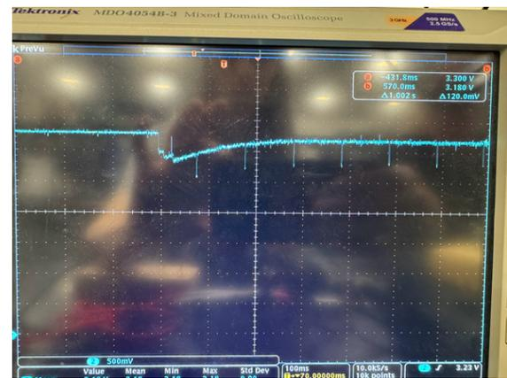
Figure 20: Oscilloscope capture at low battery
