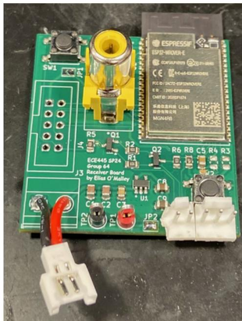
Figure 15: View of the Finished Headset Board
