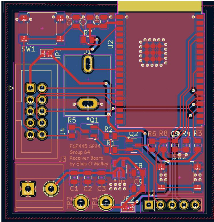
Figure 14: The Headset Board Layout
