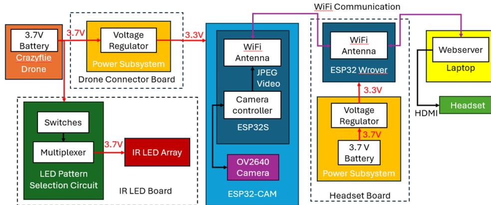
Figure 1: Functional Block Diagram for FPV Drone
