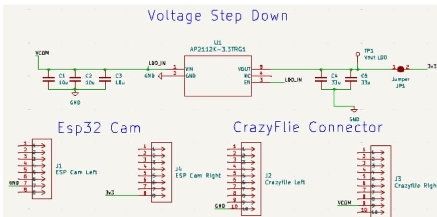
Figure 5: Schematic of the Adapter Board
