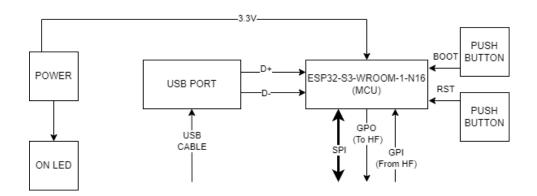
Figure 2.1: Microcontroller Board Block Diagram
