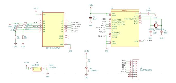
Figure 2.7: IMU Board Circuit Schematic
