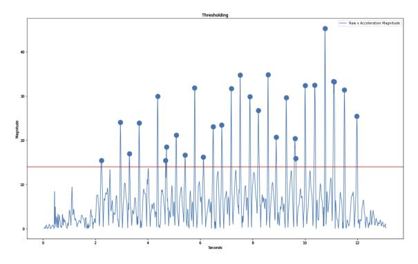
Figure 3.1: Step Detection Thresholding
