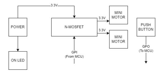
Figure 2.8: Haptic Feedback Board Block Diagram
