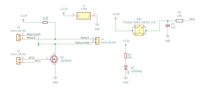
Figure 2.9: Haptic Feedback Board Circuit Schematic
