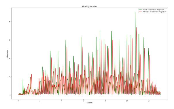
Figure 2.4: Filtered vs Unfiltered Linear Acceleration Magnitude
