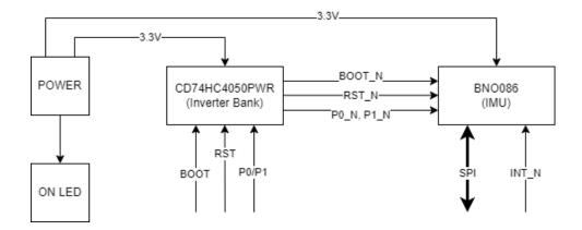
Figure 2.6: IMU Board Block Diagram
