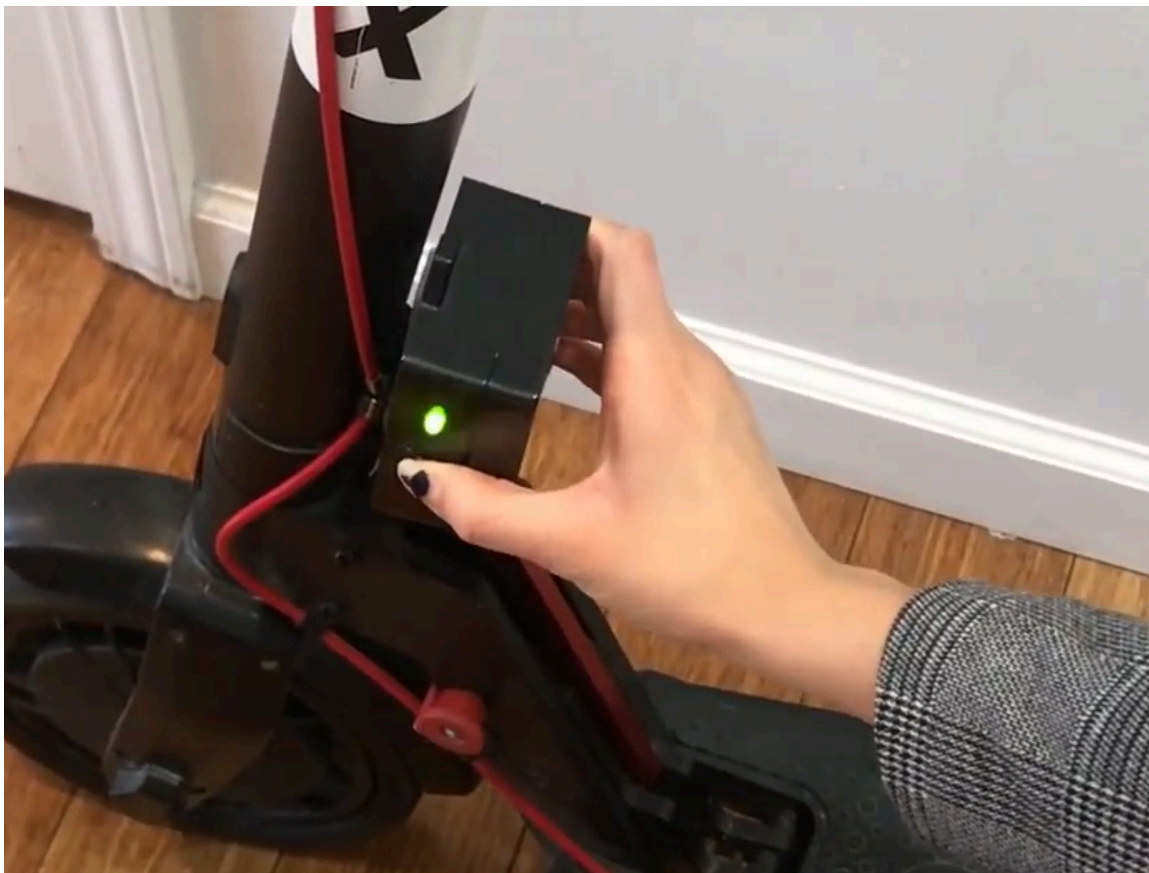
Figure B5. The LED that indicate whether the voltage for ESP32-CAM is below 4.26V
