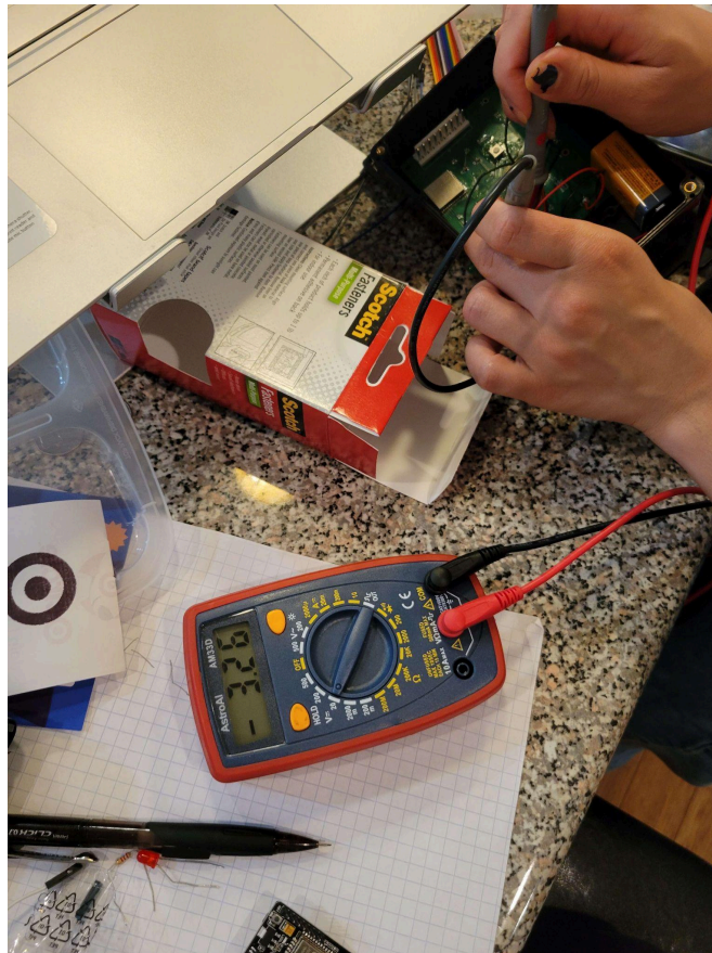
Figure B1. Voltage ESP32 supply to wire is 3.26V
