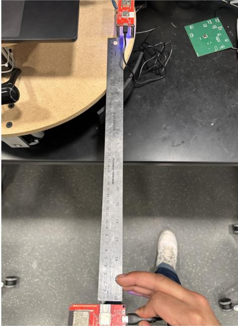
Figure 6.15: 45" Ruler between UWB Transceiver
