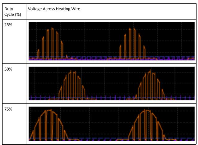
Table C.3. Recorded AC Pulse Width Modulation for concurrent heating wires(measured with oscilloscope).
