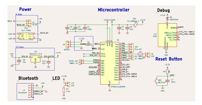
Fig. B.1. Microcontroller PCB schematic.
