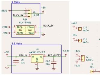
Fig. 2.3. Power subsystem on microcontroller PCB
