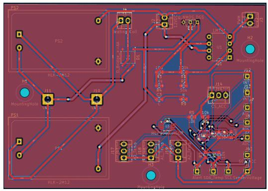
Fig. A.2. Heating coil PCB (KiCAD).
