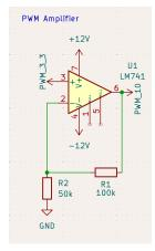
Fig. 2.6. Op-amp signal amplifier circuit.
