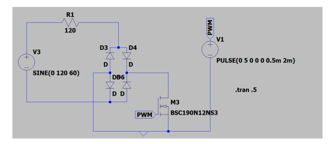
Fig. 2.7. AC Pulse Width Modulation circuit for heating coil.
