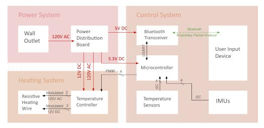
Fig. 1.2. Block diagram of overall blanket design.
