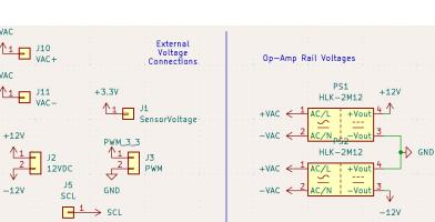
Fig. 2.4. Power subsystem on heating PCB
