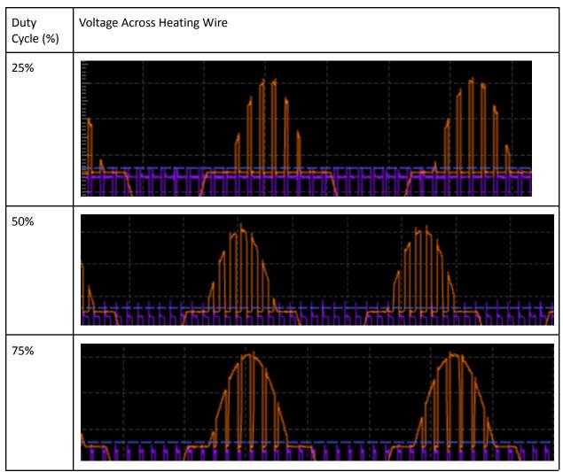
Table C.2. Recorded AC Pulse Width Modulation for individual heating wire (measured with oscilloscope).
