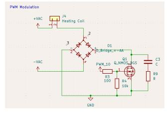
Fig. 2.5. Heating coil modulation circuit.
