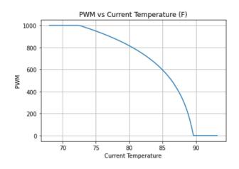
Fig D.1. PWM vs Temperature in Fahrenheit;  $T_{target}$  = 89 F.
