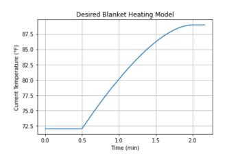
Fig D.2. Ideal heating curve over time;  $T_{\mbox{\tiny target}}$  is 89 F.
