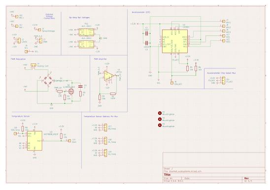
Fig. A.1. Heating coil PCB schematic.
