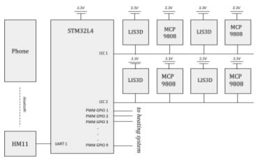
Fig. 2.1. Block diagram of control system.
