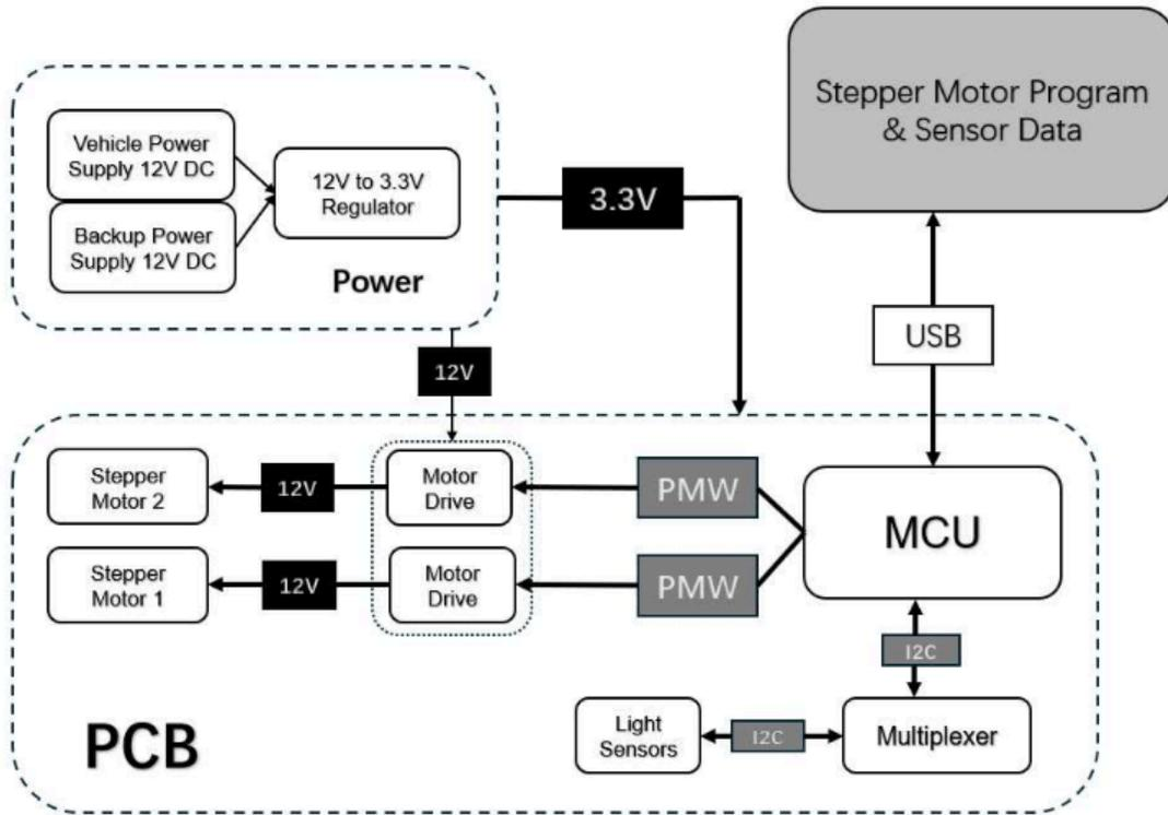
Figure 4: Block Diagram
