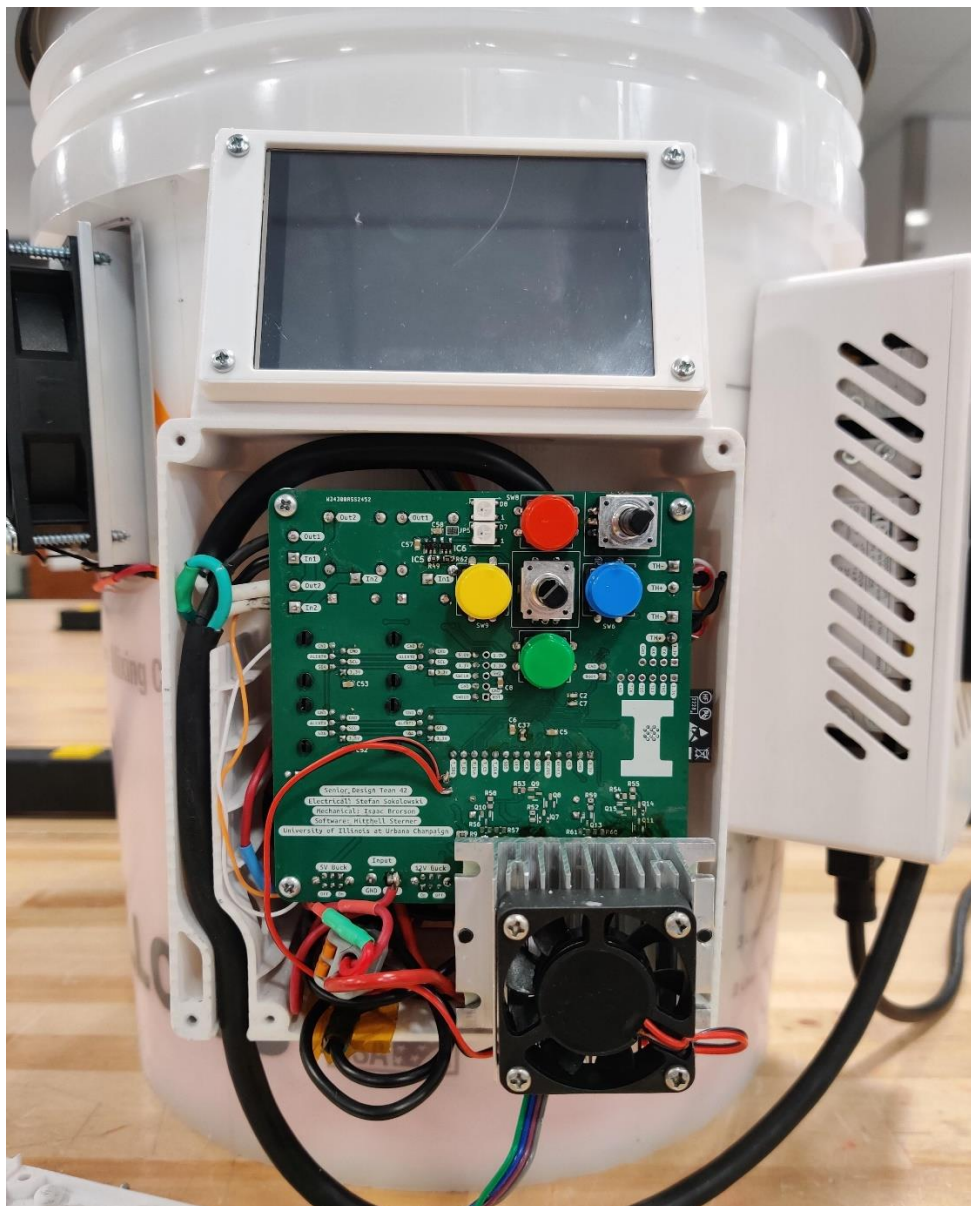
Figure C.2.3: Assembled PCB with Heatsink in Enclosure
