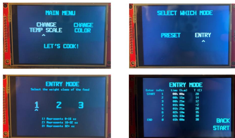
Figure 4: Various Setup Phase Submenus
