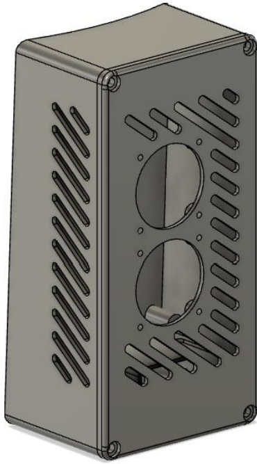
Figure B.1.1 Power Supply Ebox 3D Design and Finished Print
