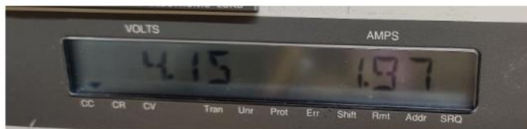
Figure C.4.1: Power Subsystem Verification on Programmable Load
