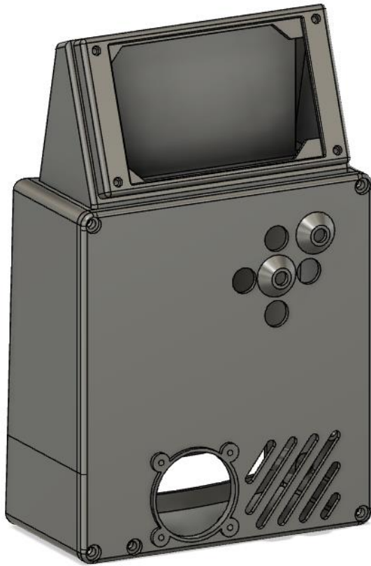
Figure B.2.1: Main Board Ebox 3D Design and Finished Print
