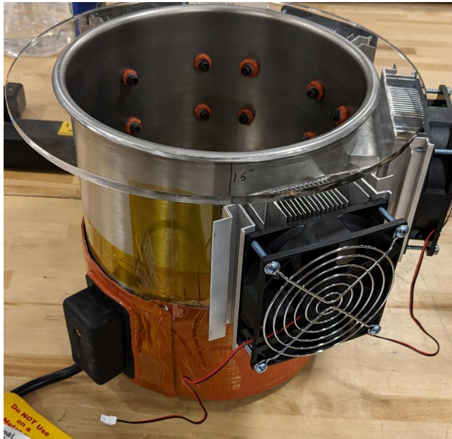
Figure B.3.1: Heating Band Placement
