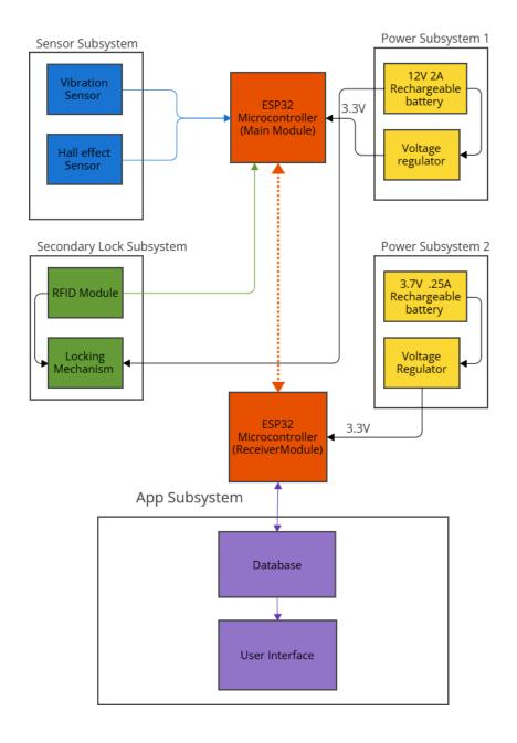
LEGEND: Green: I2C connection Blue: GPIO Connection Orange: ESPNOW data transfer Purple: Bluetooth Connection
