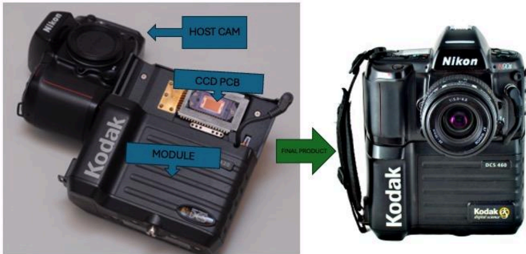
Fig. 1: High level implementation of solution depicting old camera to be harvested and the final product that our solution would resemble. Please note that our solution would be a lot more compact than the depicted model
