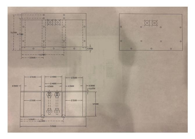
The body will be primarily made out of Medium Density Fibreboard (MDF), with the front and back face being made out of metal so as to be more easily drilled through.
