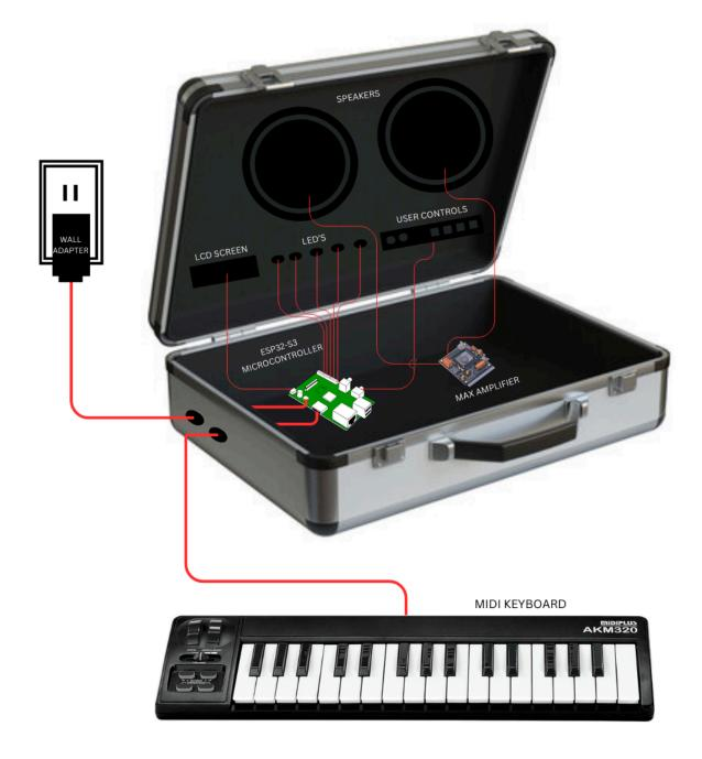
Figure 1: Visual Aid of the Virtual Synthesizer
