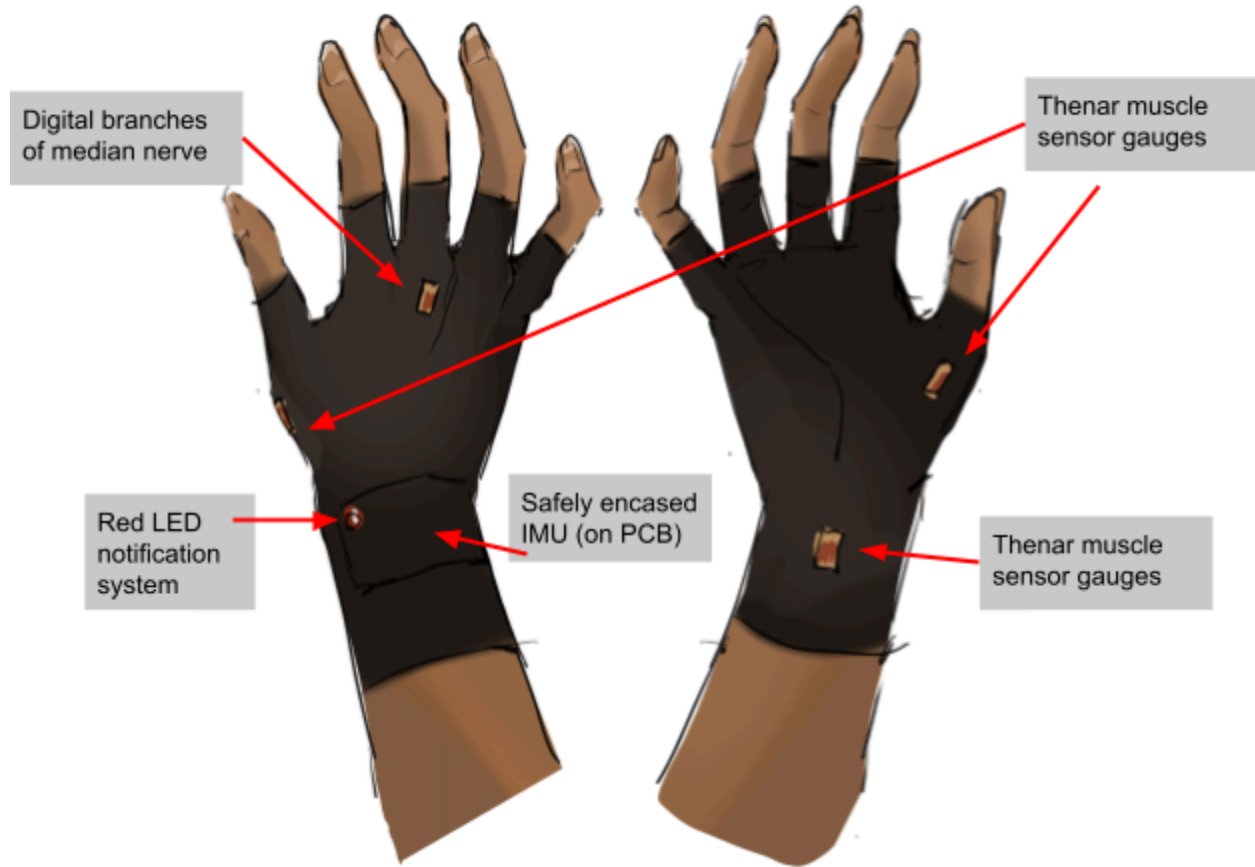
Figure 3: Physical design & sensor placement
