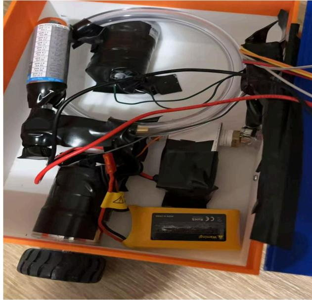
**Figure 2.** This is a picture of how our actual Battlebot was laid out. There are two motors towards the backside of the internal layout of our Battlebot. To control these two motors, we mounted our H-Bridge on the front wall of our Battlebot. The reasoning of using a different H-Bridge will be discussed later in *Section 2.1 Drivetrain*.
