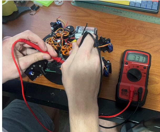
Figure 13 3.3V output from linear regulator
