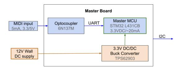
The Master Board will be composed of three parts: an optocoupler, the master MCU, and an integrated 3.3V DC/DC converter.
