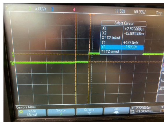
Figure 6: Stable 3.3V Waveform
