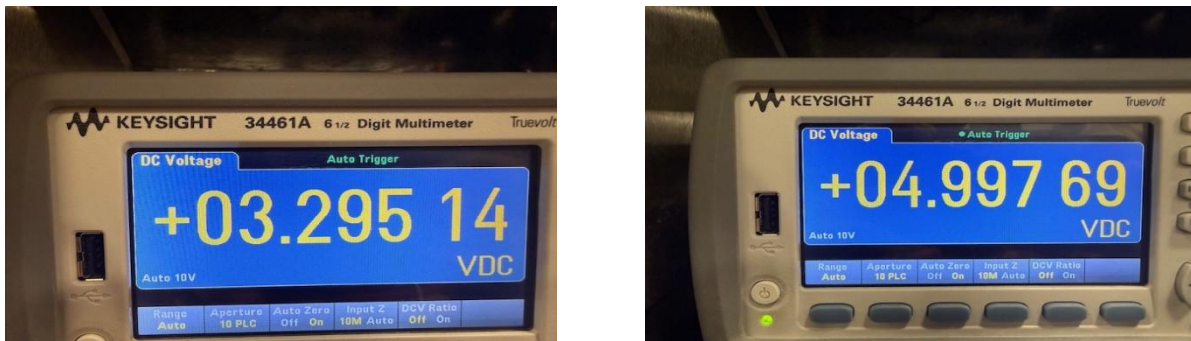
Figure 8 5V and 3.3V readings
