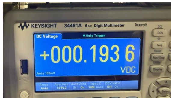
Figure 11 Voltage reading at FB Pin for 100% Duty Cycle
