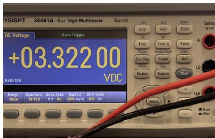
Figure 10: Multimeter Measurement on 3.3-Volt Linear Regulator Output
