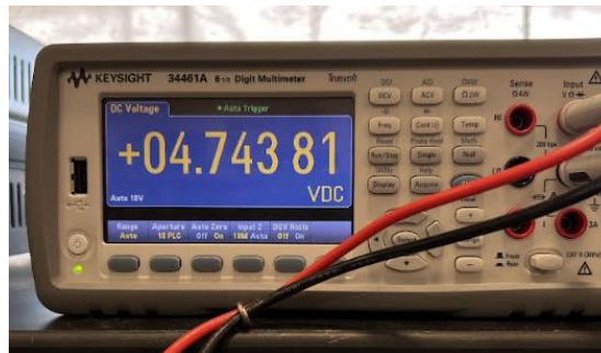
Figure 12: Multimeter Measurement Across Motor With a Low Safety Signal
