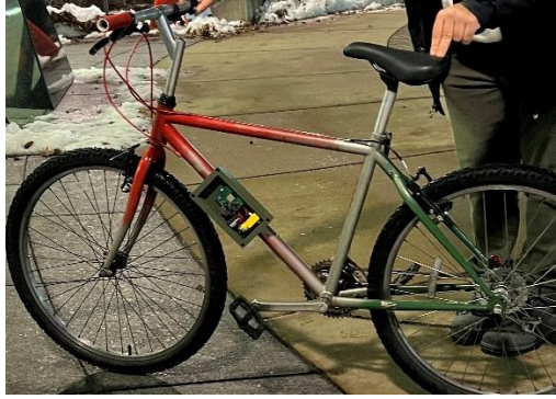
Figure 2: Our e-bike crash detection and safety system housed in an enclosure, mounted on a test bicycle
