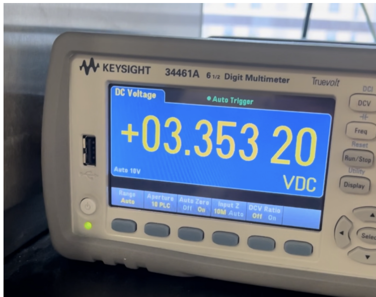
Figure 8: 3.3V Buck output reading via DMM showing 3.353V output.
