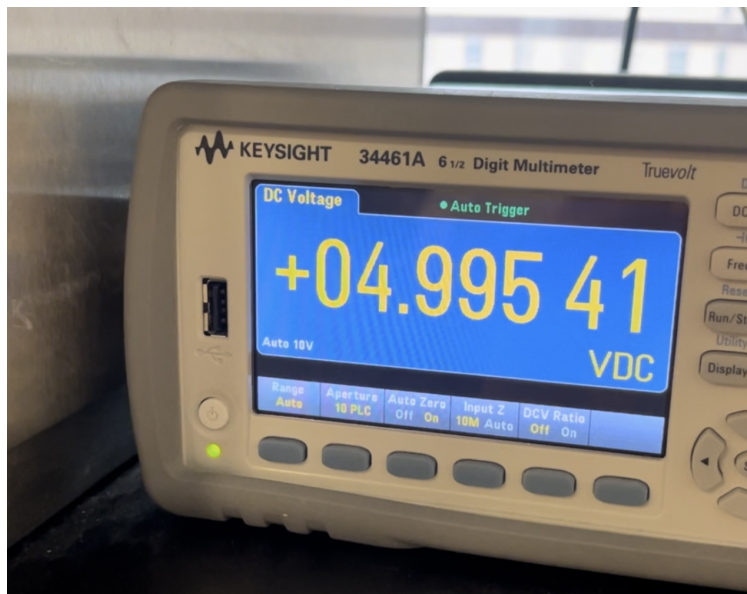
Figure 9: 5V Buck output reading via DMM showing 4.995V output.
