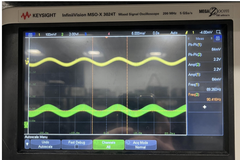
Figure 7: Pre and Post amplification piezo signal on oscilloscope. Channel 1 (yellow) shows raw piezo signal ( \sim 84\text{mV} ), Channel 2 (green) shows amplified output ( \sim 2.2\text{V} p-p).
