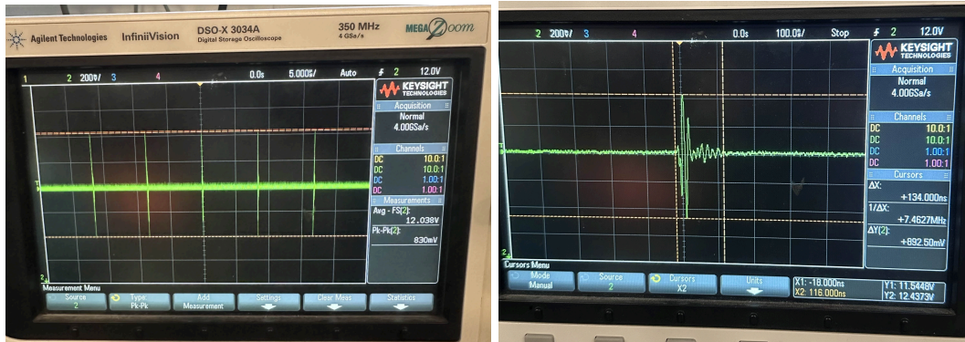
Figure 20: +12 VDC output (left) and zoomed in on the high frequency ringing (right)
