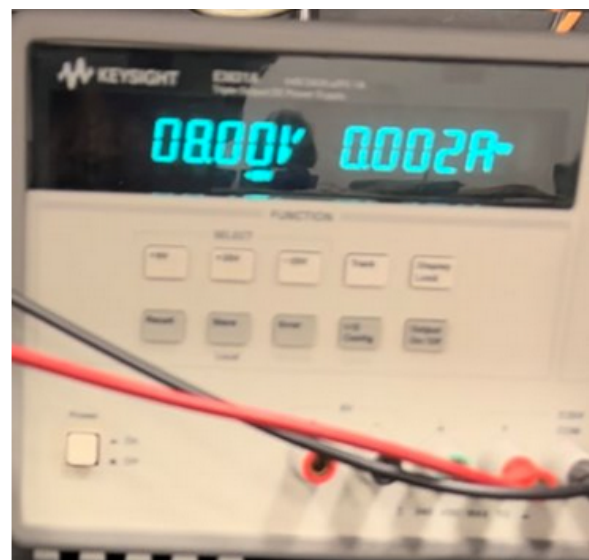
Figure 16: Charging with 8V across USB-A V_{bus} and ground records a 4.14V potential difference across the battery terminals to allow constant voltage charging
