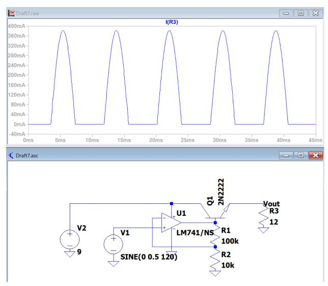
Power amplifier design using BJT at output to drive higher current- should use a complementary pnp to pull some current as well on negative half cycle
