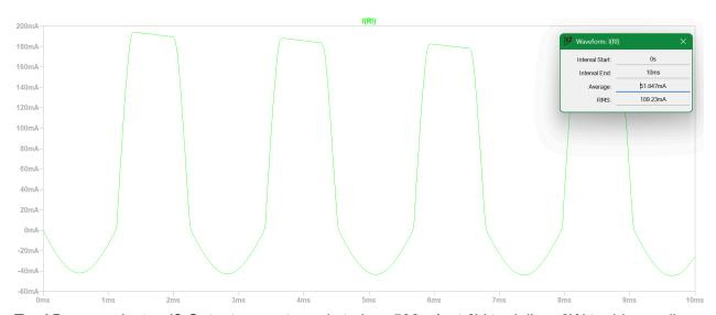
Try AB opamp instead? Output current needs to be ~500mA at 6V to deliver 3W to driver coil
