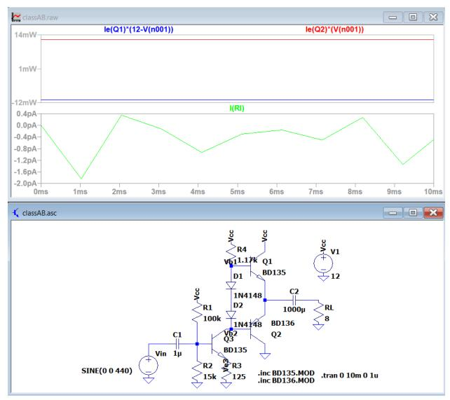
Max loss at  $\sim 350 \text{mW}$  for both BJTs, this shouldn't be too much heat, when both off power consumption is < 20 mW
