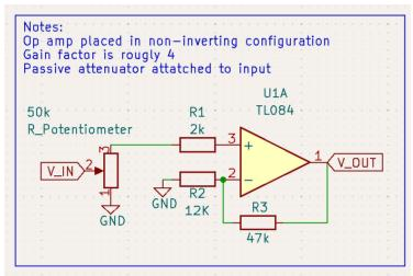
This will be tested in the upcoming week as all parts are sourceable from the ECE supply center Testing can be conducted with a guitar and an oscilloscope, ensuring the correct relationship between v\_out and v\_in from the signal of a guitar pickup.
