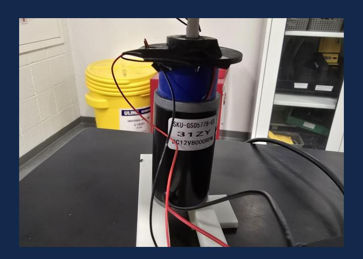
We utilized a 31ZY motor. While this motor has little torque, it is perfect for this design due to its high amperage rating (2 Amps), high voltage maximum (12 Volts), and maximum spin speed (6000 RPM).
