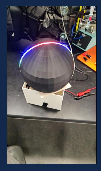
Due to the mechanical mishaps with our current design, we are unable to spin our device up to the desired speed of 600 RPM. However, the following video demonstrates our designs speed ability of 120 RPM.
