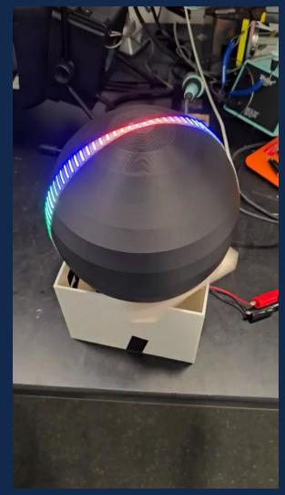
As shown, our LED array is powered externally while spinning. This is indicative of properly transferring power from a stationary to spinning reference frame.
