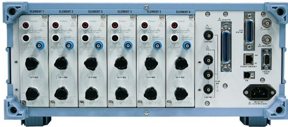
Yokogawa WT1800 High Performance Power Analyzer ($10,000+)
