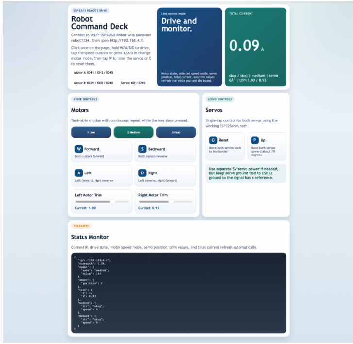
Figure 4: Operator interface used for wireless command input, drive tuning, and monitoring.
