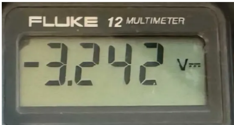
Figure 6: Regulator Output Voltage
