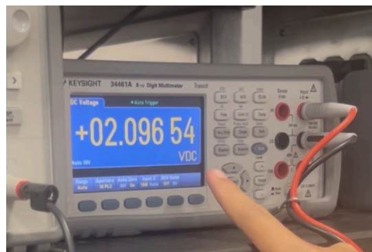
Figure 11 - 50V_{DC} to 2V output
