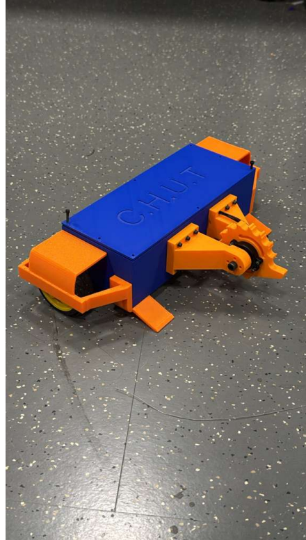
Figure 4: Final assembled C.H.U.T. battlebot with printed chassis, lid, skids, wheel protectors, rear wheels, and front spinner assembly.
