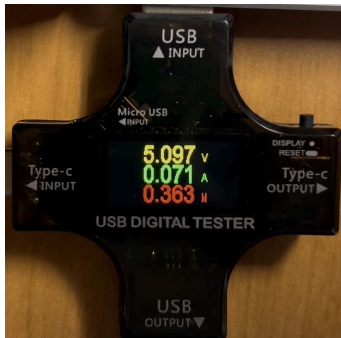
Figure 9: Multimeter measurements of power supply
