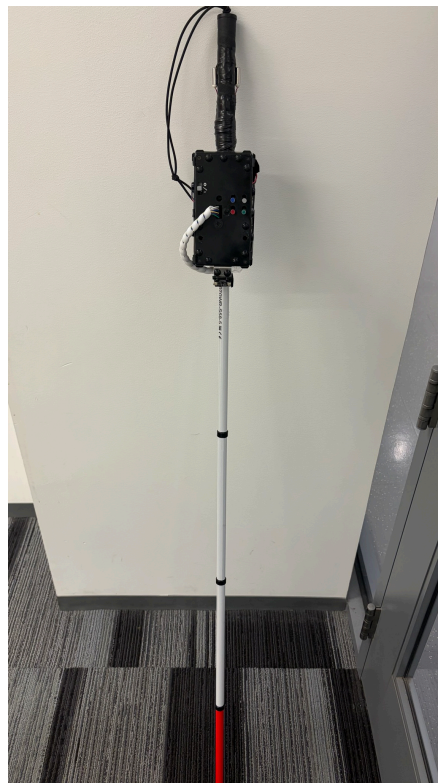
Figure 1: The completed SafeStep prototype mounted on a standard white cane.
