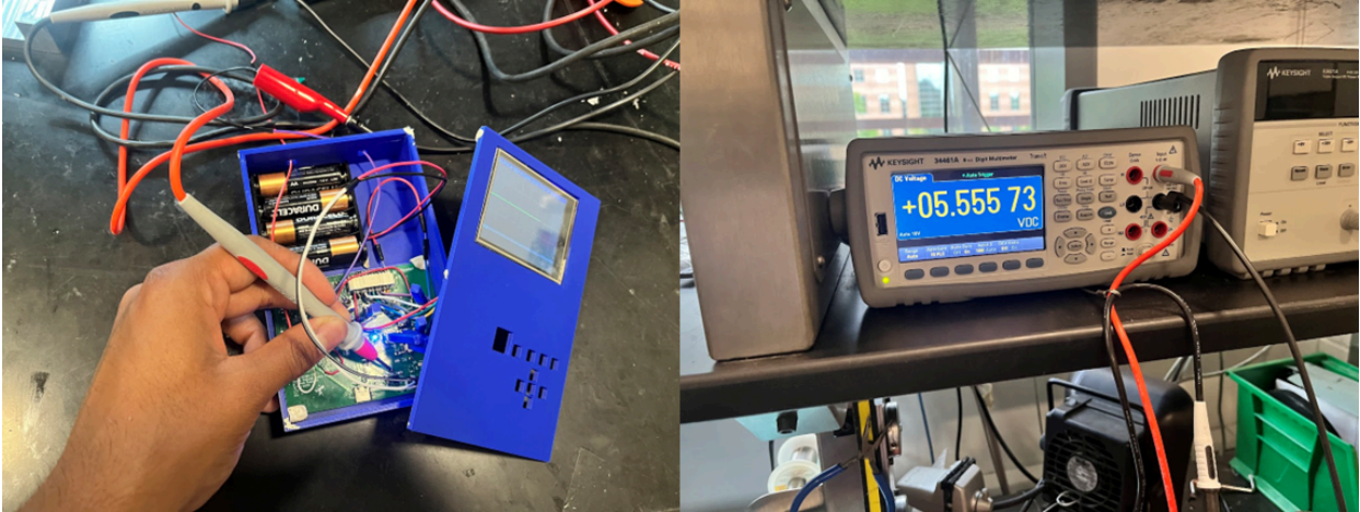
Figure 7. Battery pack voltage after protection diode
