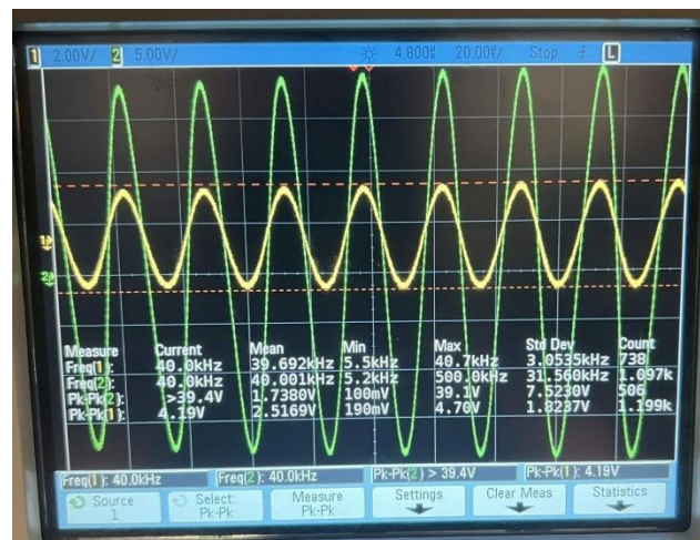
Figure 12 Pre-amplification (channel 1) and post-amplification (channel 2) signals
