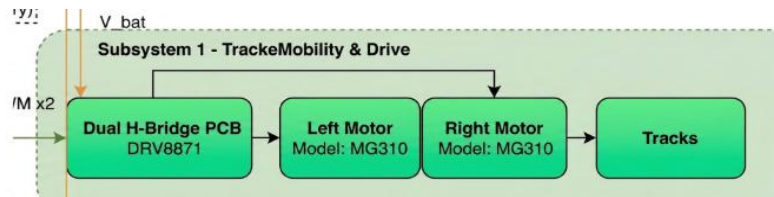
Figure 4: Block Diagram of Subsystem 1
