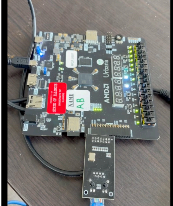
Figure C.18. Bench setup (referenced from §1.3): Spartan-7 Urbana board with the LAN8720 PHY module on Pmod B, Ethernet cable to the host, and USB programming/UART link.
